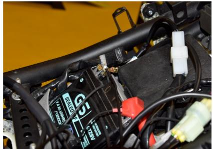
Connect the Pink ARA wire to the Yellow/Black wire of the Clutch switch behind the clutch lever.
