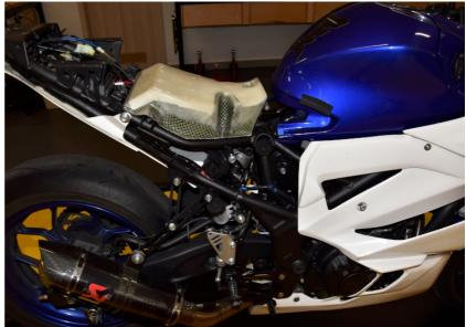
On this photo the ARA used together with the iQSE quickshifter. The iQSE plugs should always be the last in the chain i.e. connected directly to the ignition coil plugs.
