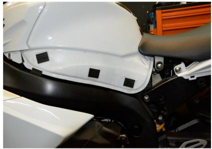
Remove the cover from the tank on the right side.
