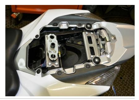
Remove the cover from the tank on the left side.
