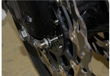
Connect the 3-pole sensor connector to the ARA wiring.
